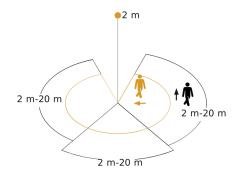
Possible mounting height: 2,00 m - 5,00 m Orange: radial Black: tangential 3 scalable zones
